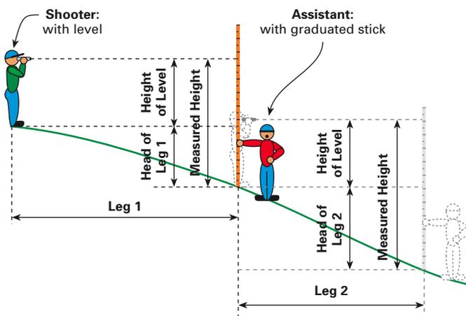
1. Subtract height of level from measurement on stick to determine head for each leg.
