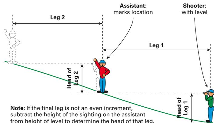
**Note:** If the final leg is not an even increment, subtract the height of the sighting on the assistant from height of level to determine the head of that leg.
