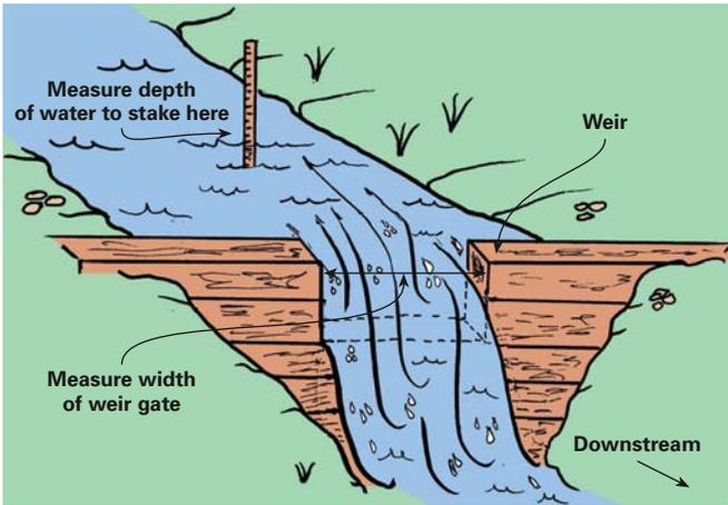
**Step 2.** Compute the area of the cross-section you just measured by multiplying the average depth you just computed by the width of the stream. For example, a 6-foot-wide stream with an average depth of 1.5 feet would yield a cross-sectional area of 9 square feet.
